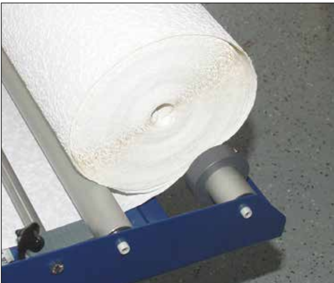
3.2. Inserting a roll of wallpaper, adjust the guide roller to the width of the roll
