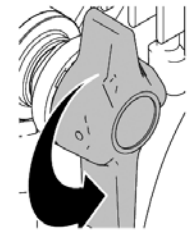
Valve opened (ventilation & pressure relief)
