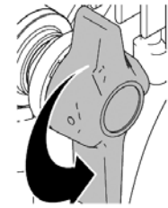
Valve open (ventilation & pressure relief)
